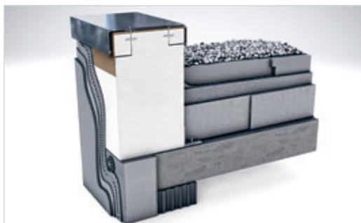
With integrated plastic strips for attaching the flashing
